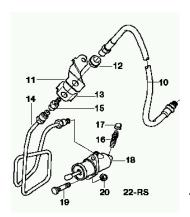
**PLEASE NOTE-** Some late model BMW vehicles are factory equip with a clutch delay valve, or "Lock Valve" (see diagram- item #15) located in the clutch hydraulic line between the master and slave cylinders. This valve is designed to provide a controlled clutch engagement for a smooth "drive-away" by metering the return flow rate of hydraulic fluid from the slave cylinder to the master. The net effect is that the clutch "engagement rate" is slowed and not directly controlled by the driver.
